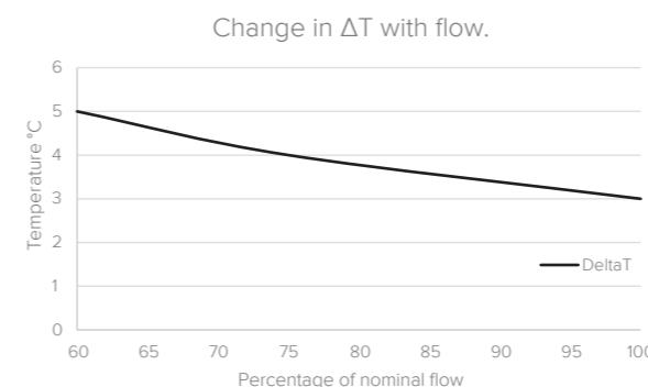
The diagram shows when  $\Delta T$  is at 3°C, as the power and COP of the heat pump are at 100%. When  $\Delta T$  increases to 4 degrees, the C.O.P. drops by 1.5% and power drops by 3%. When  $\Delta T$  reaches 5 degrees, the COP drops by 4% and power drops by 6%. Note that a  $\Delta T$  of 4 degrees is still acceptable, but any higher will negatively affect the heat pump's performance.
