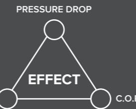
A LOW PRESSURE DROP IS ESSENTIAL FOR THE GEOTHERMAL ENERGY SYSTEM TO WORK EFFECTIVELY. IF THE PRESSURE DROP IS TOO HIGH, THIS LEADS TO A WORSE  $\Delta T$ , C.O.P. AND POWER IN THE HEAT PUMP.
