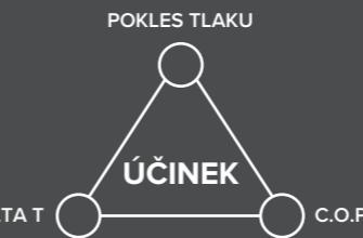
**PROVOZ SYSTÉMU GEOTERMÁLNÍ ENERGIE S POŽADOVANOU ÚČINNOSTÍ VYŽADUJE NÍZKOU HODNOTOU TLAKOVÉHO POKLESU. JESTLIŽE BUDE TLAKOVÝ POKLES PŘÍLIŠ VYSOKÝ, POVEDE TO K HORŠÍM HODNOTÁM ΔT, C.O.P. A VÝKONU TEPELNÉHO ČERPADLA.**
